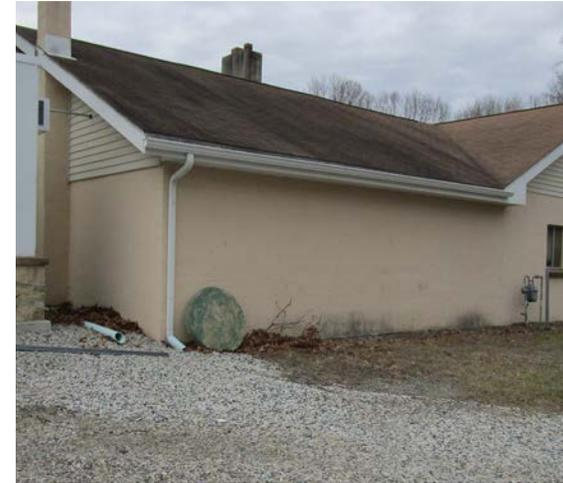
Two rain gardens can be installed near the building to capture runoff from the building. These systems can easily be incorporated into existing landscapes, improving aesthetics and creating wildlife habitat while managing stormwater runoff. A preliminary soil assessment suggests that the soils have suitable drainage characteristics for green infrastructure.
